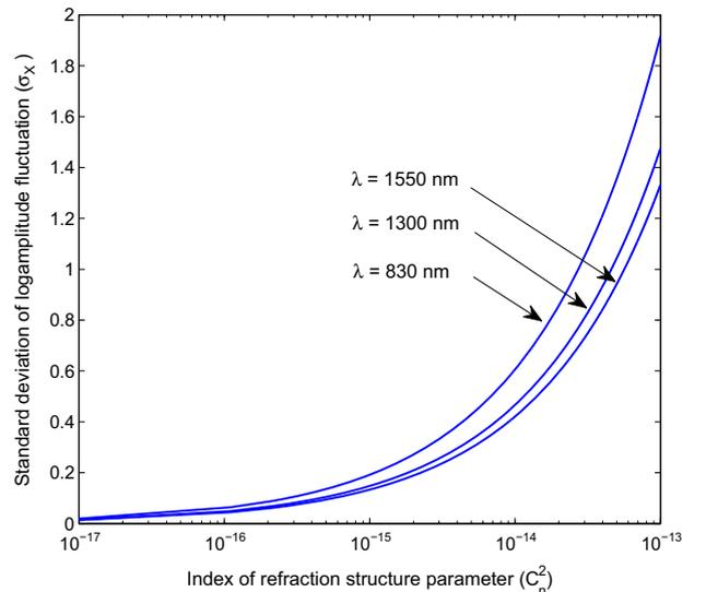
**Fig. 2.** Standard deviation of log-amplitude fluctuation ( $\sigma_X$ ) versus index of refraction structure parameter ( $C_n^2$ ). The wavelengths are 830 nm, 1300 nm, and 1550 nm, respectively. The propagation distance is 2 km.
