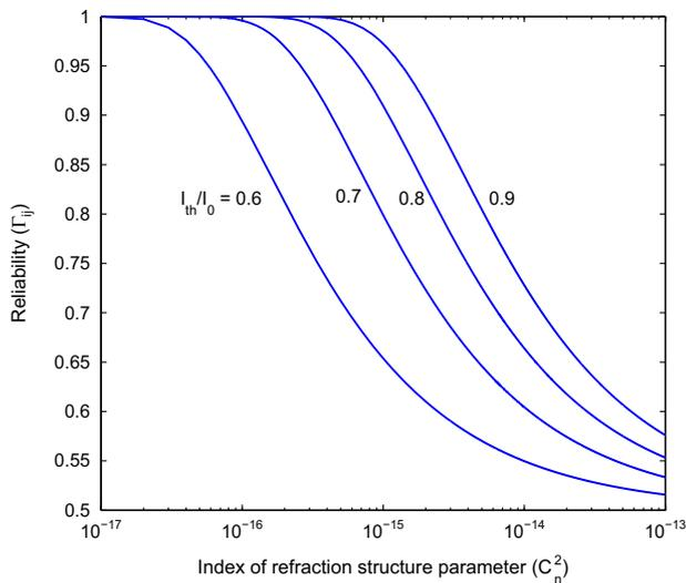
**Fig. 3.** FSO link reliability ( $\Gamma_{ij}$ ) versus index of refraction structure parameter ( $C_n^2$ ). The wavelength is 1550 nm on the 2 km path. The ratios of  $I_h/I_0$  are 0.6, 0.7, 0.8, and 0.9, respectively.
