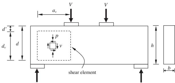
Fig. 3. Concrete stresses within shear span of a deep beam.
