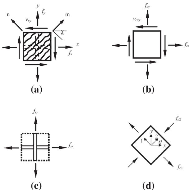
Fig. 1. Stresses of cracked reinforced concrete membrane elements subjected to shear. (a) Cracked reinforced concrete membrane; (b) concrete membrane; (c) steel reinforcement; (d) principal angle and stresses.
