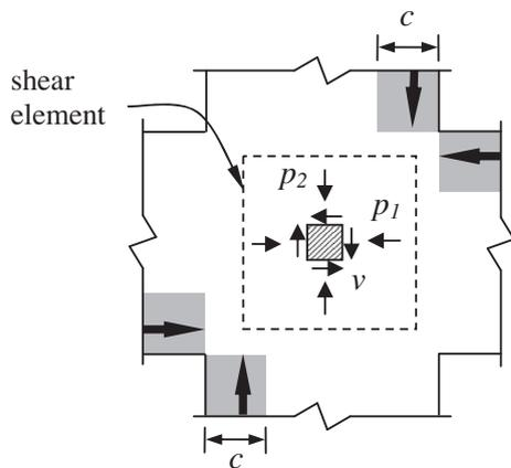
Fig. 4. Stresses in an interior beam–column joint.
