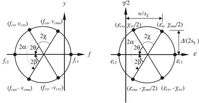
Fig. 2. Mohr circles of average stress and average strain for cracked concrete.
