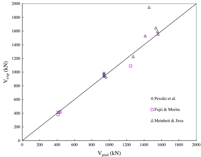
Fig. 8. Correlation of experimental and predicted joint shear strengths.
