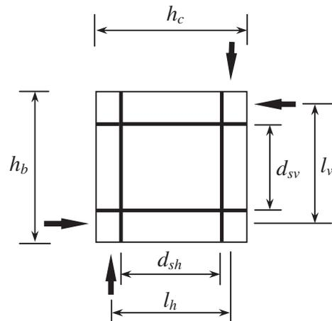
Fig. 5. Dimensions of an interior beam–column joint.
