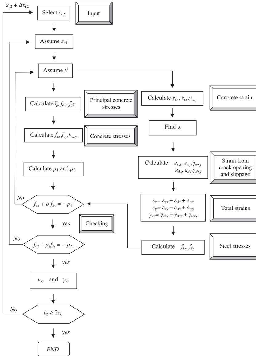
Fig. 7. Flow chart of computational solution procedure for determining shear stress–strain relationship of RC interior beam–column joints by MRA-STM.
