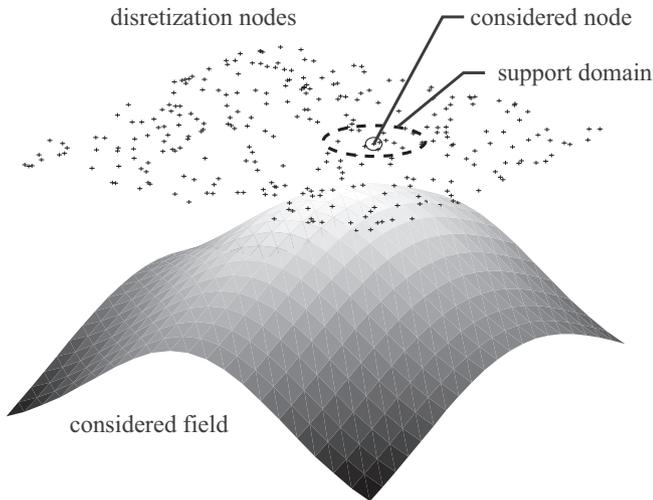
Fig. 2. Schematic representation of the meshless numerical principle.
