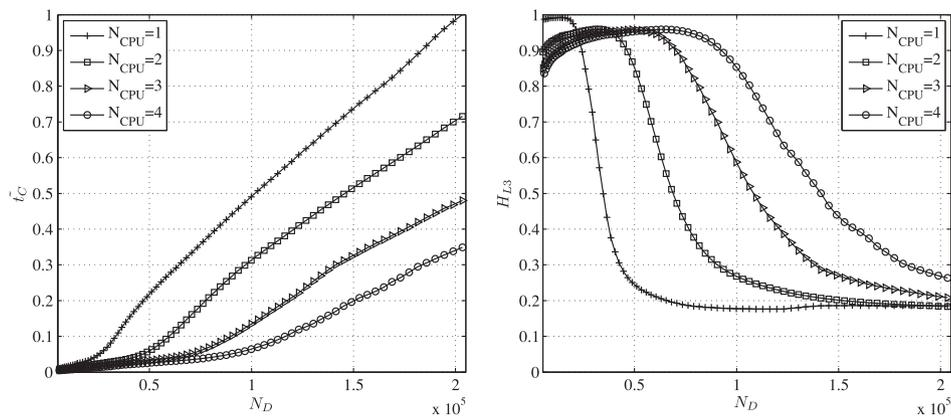
Fig. 9. Computation time (left) and L3 cache hit rate (right) with the respect to the number of discretization points and the number of CPUs.
